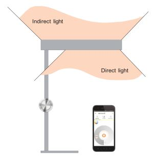
The floor-standing luminaire can be switched and dimmed with one pushbutton.
