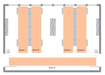
The open-plan office luminaires are floor-standing luminaires in the desk area and downlights in the corridor area. They are divided into five light zones.
