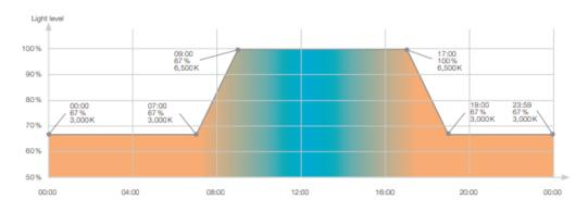
HCL will start automatically with default settings after synchronizing the real-time clock. Automatic sync done by connecting with the DALI CONFIG APP.
