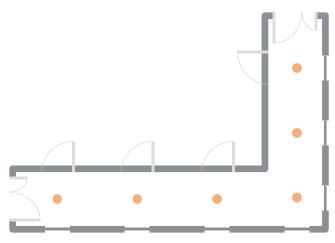
The lights will be switched on automatically when a person enters the corridor and automatically dimmed down to a light level of 10 % after the delay time has expired and if no presence is detected.
