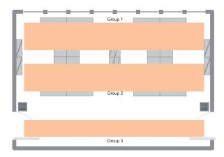
The open-plan office luminaires are divided into three light groups which can be switched and dimmed.
