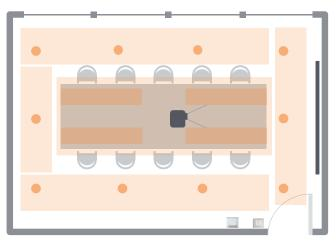
The meeting room luminaires can be switched and dimmed and pre-configured. Light scenes can be recalled by using pushbuttons.
