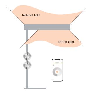
The floor-standing luminaire can be switched and dimmed with two pushbuttons.
