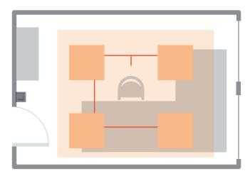
The office luminaires can be switched and dimmed with one pushbutton.
