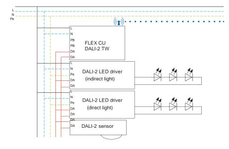
b) Wiring diagram of group 1 with standard DALI luminaires
