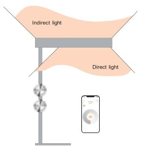
The floor-standing luminaire can be switched, dimmed and tuned (Tunable White) with two pushbuttons.
