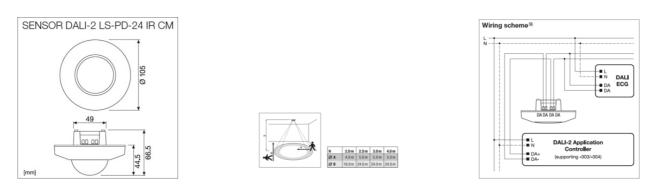
April 28, 2025, 20:01:30 SENSOR DALI-2 LIGHT/PRESENCE-24 INFRARED CEILING MOUNTING
